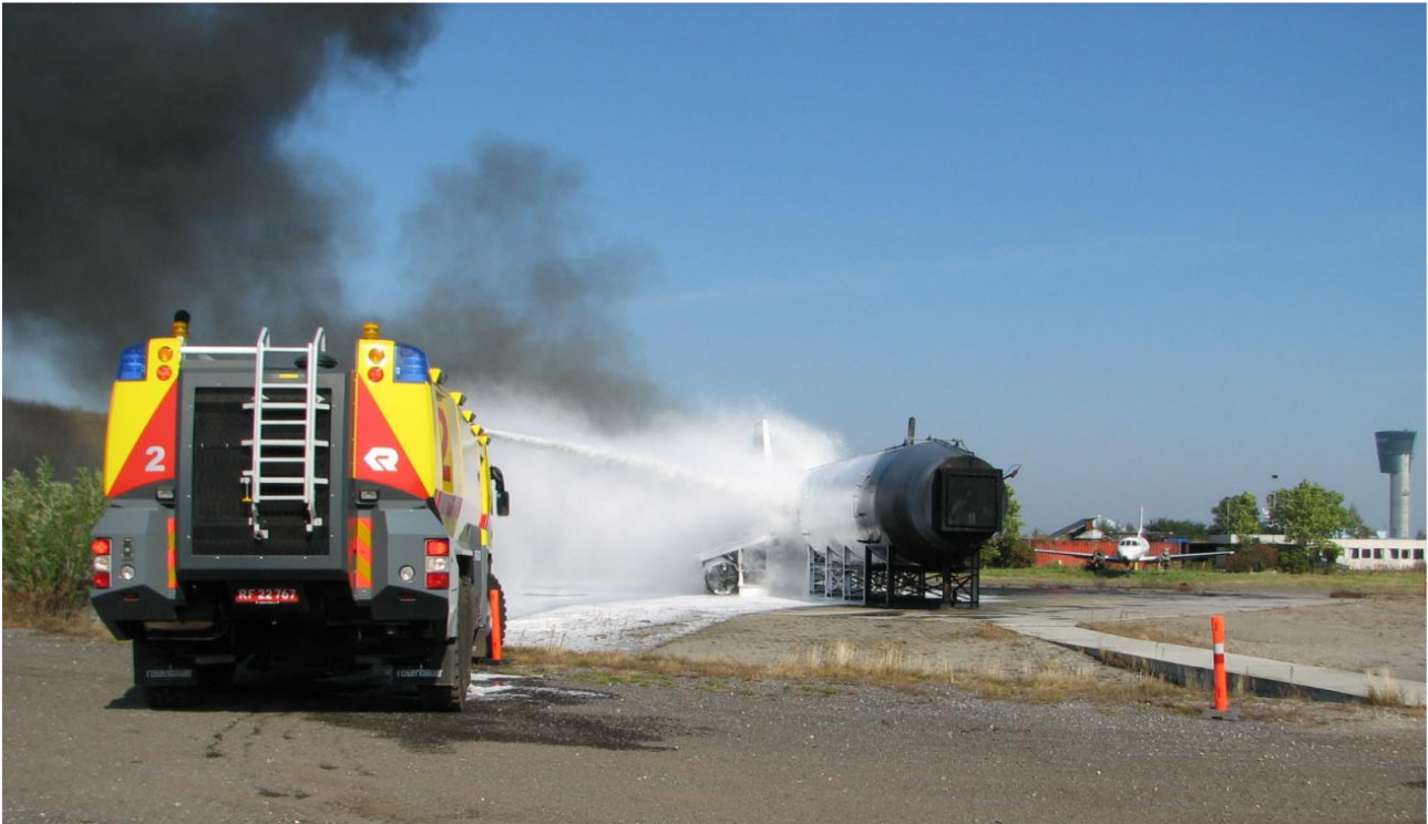
Figure 7.1 Training at Copenhagen airport with crash tender. Picture courtesy of Kim T. Olsen, Copenhagen Airports A/S. ( https://beros.dk/skum/Kim_Thorbojern_Olsen_CPH.pdf ).
