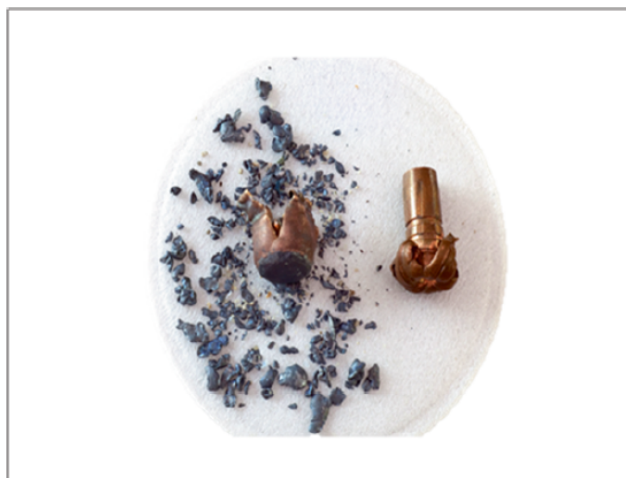
Figure 1-25: Lead fragments from a copper jacket lead-based bullet (left) compared with a copper expanding bullet (right) after Golden et al. (2016)
