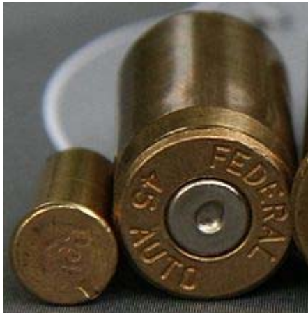
Figure 2-9: Calibre markings on the bottom side of a cartridge case (right) and the bottom side of a rimfire cartridge (left), also showing for centrefire ammunition the place of the detonator in the centre of the bottom side of a cartridge
