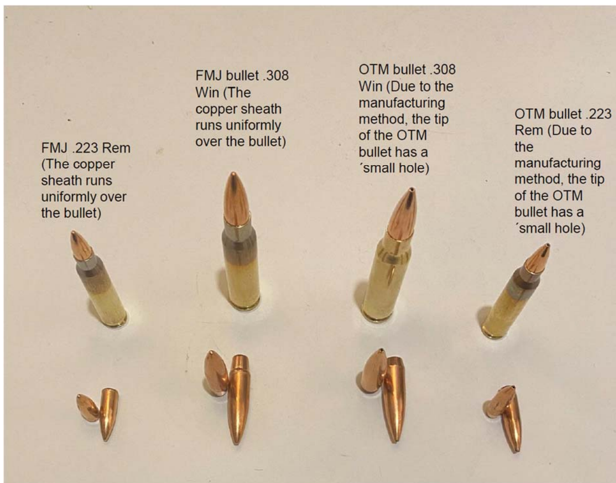
Figure 2-12: Exterior characteristics FMJ and OTM bullets
