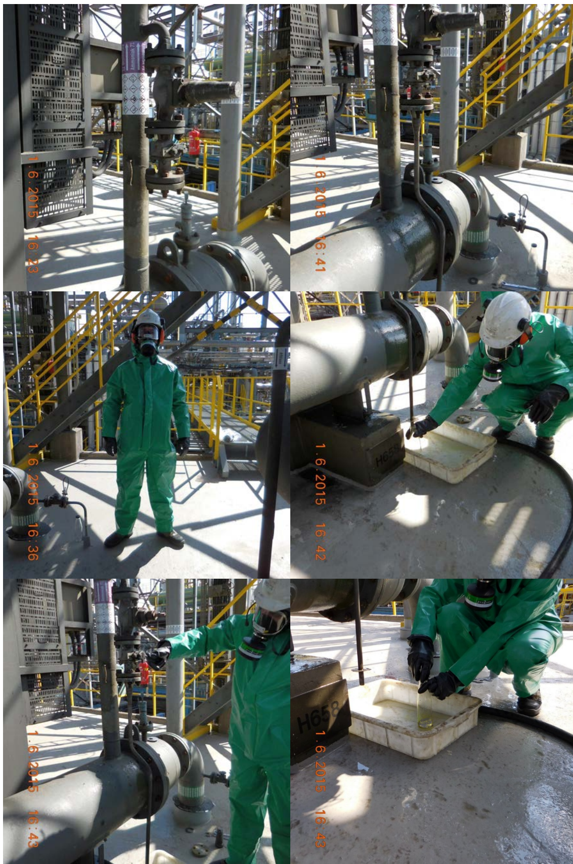
Figure 4: Sampling procedure (simulated realistic use conditions). Sampling point in regular state; sampling point with installed pipe; worker with prescribed PPE; placing of sample bottle; opening of valve; removal and sealing of sample bottle (from upper left to lower right).
